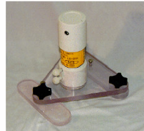
Figure 7: A single STROAB beams a vertically spread laser signal while rotating at 3,000 rpm. (Courtesy of MTI Research)
